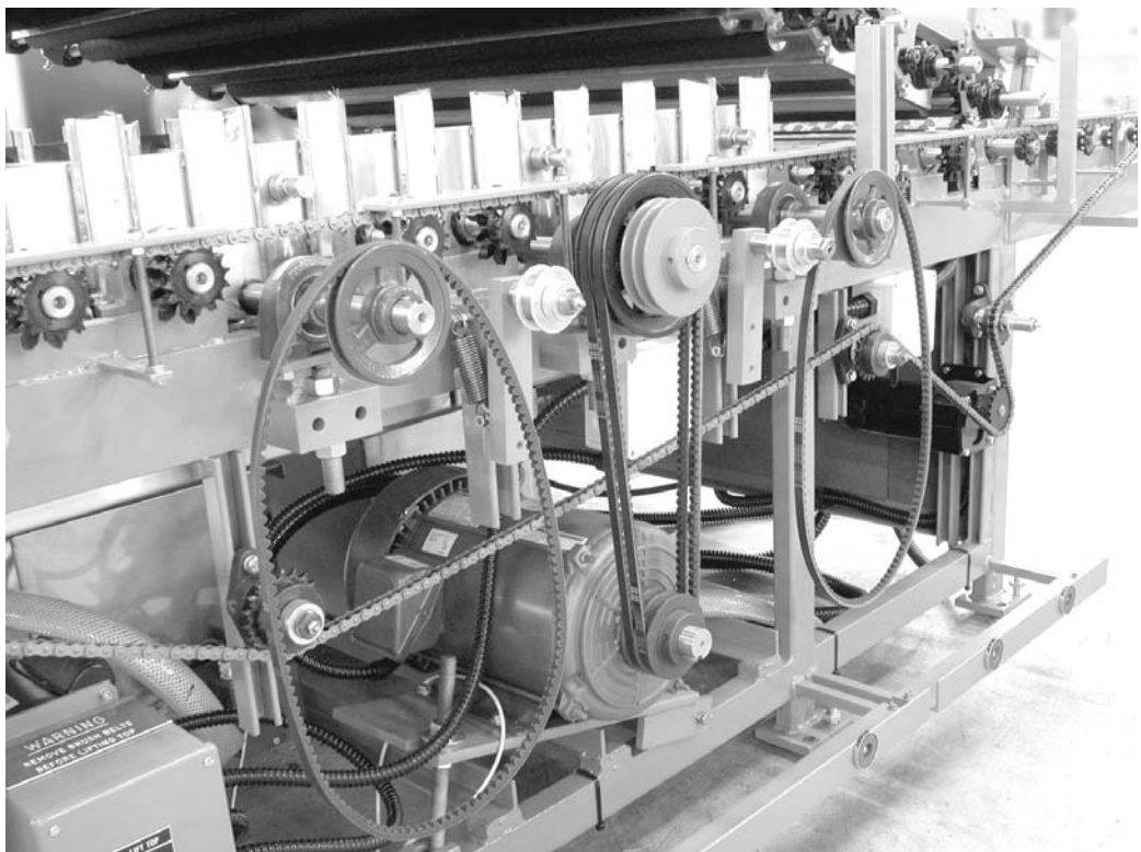
BELTS REMOVED TO RAISE UPPER SECTION
