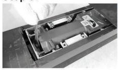
Depending on the application, adjust the closing power of the closer using the screw 7.
