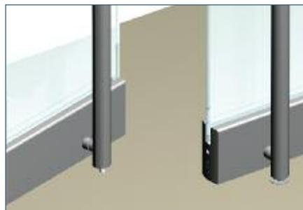
Rail Mount Detail at Latch at Floor With AMR209PS Dustproof Keeper
