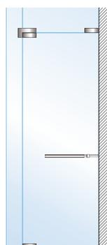
Single Door Installations Require One Locking Ladder Pull and a Dustproof Keeper
