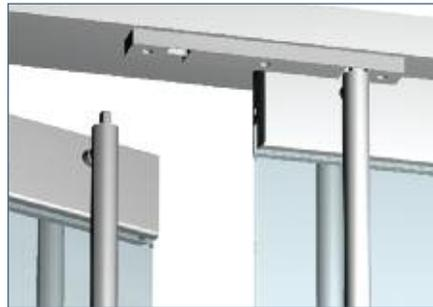
Rail Mount Detail at Latch With Header and PK Strike
