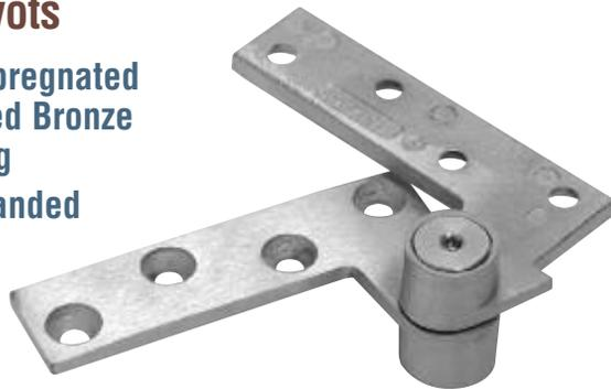
These Offset Top Pivots are supplied with an oil-impregnated sintered bronze bearing, and intended for use with standard aluminum, wood, and hollow metal doors. These Pivots are fully mortised and non-handed. They are supplied with wood and machine screws to allow most common installations.
