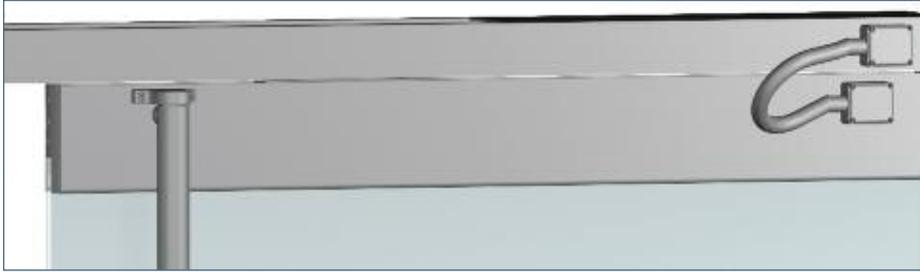
Rail Mount Detail at Header and Wire Loop for EG100
