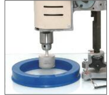
Swivel the head to one side for drilling larger holes up to 6" (152 mm)
