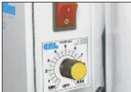
Electronic Variable Speed Control
