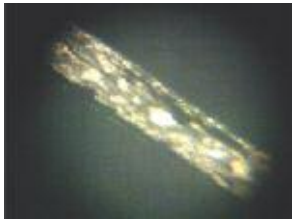
LIGHT SURFACE or SCUFF MARK SCRATCH – Over 95% of all scratches are light scratches or scuff marks. This magnified image above shows a light scratch. This scratch can be removed.
