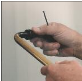
Remove existing handle or knob and discard.
